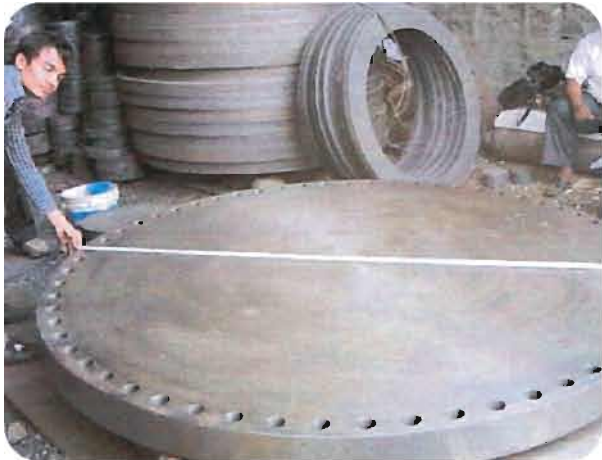
Visual & Dimensional inspection in progress
