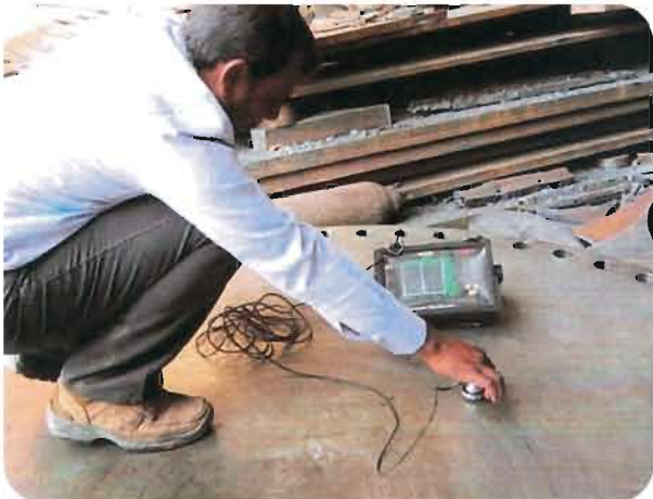
UT test witness in progress
