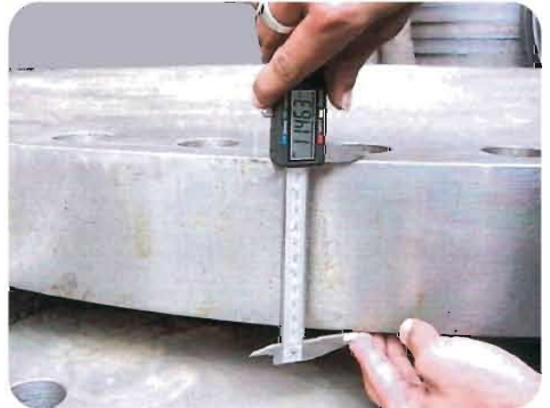
Visual & Dimensional inspection in progress
